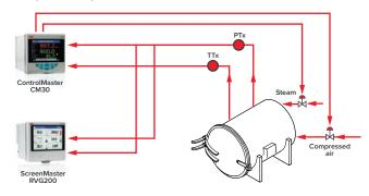
ABB's paperless recorders, protected to NEMA 4X and IP66 as standard, are used to record critical process parameters such as temperature, pressure and door open or close signals. Also the batch recording option in ScreenMaster enables data, including batch numbers and product type information, to be recorded alongside process data. With ABB's DataManagerPro software, collected batch records can be displayed rapidly by searching for their batch number or batches with common attributes identified.
